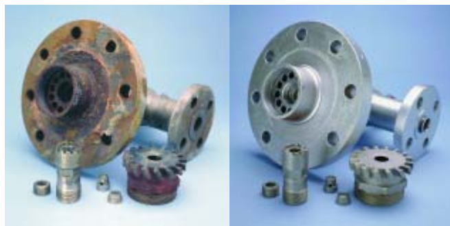
FIG. 4. A disassembled fuel nozzle before (left) and after (right) refurbishment.
