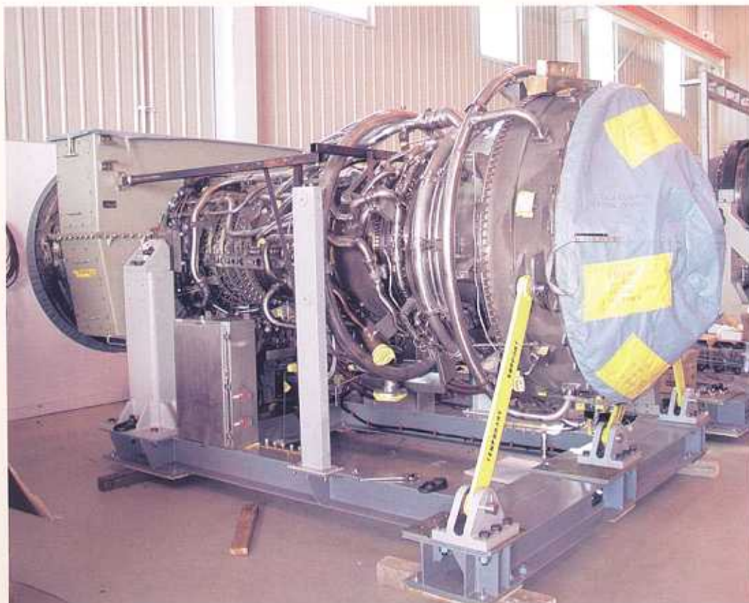
Twelve-hour swap. Specialized quick disconnects, engine crane and monorail handling systems allows test engineers to remove, reinstall and align an LM6000 for weekend full load testing using standard cold end drive and producing MWs at a functioning power plant site installation.
